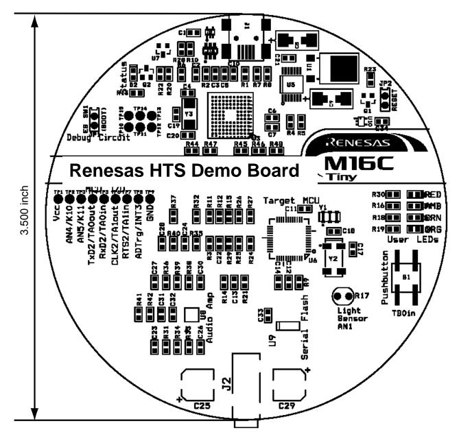
Figure E-1: PCB Top View
